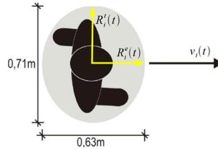
**Fig. 1.** Mean Elliptical Motion Range of a Pedestrian [6]
