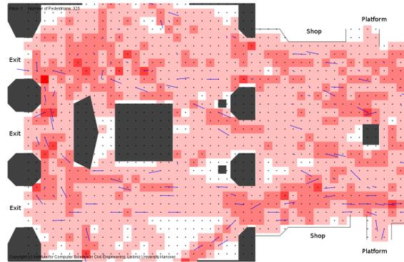
Fig. 7. Hanover Central Station - Density and Velocity with JWalkerS
