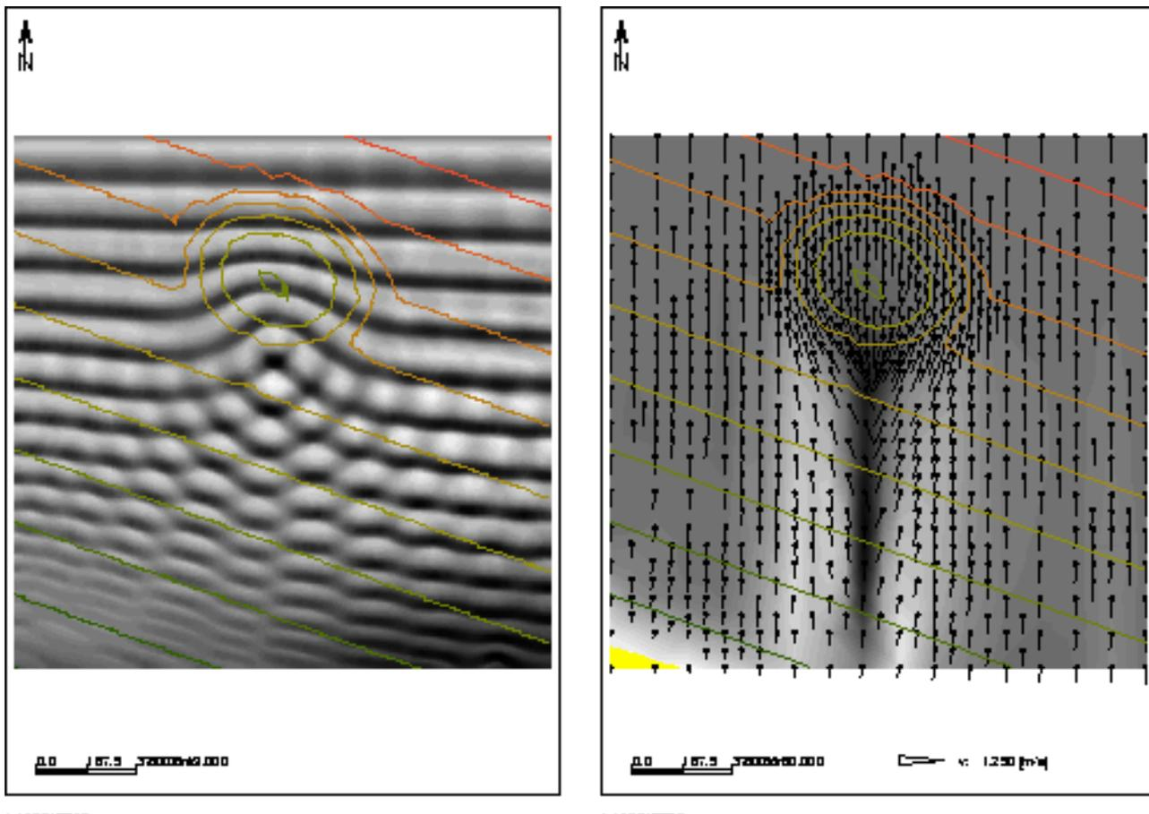
**Figure 1:** Results from an inter-period and a hyperbolic wave model
