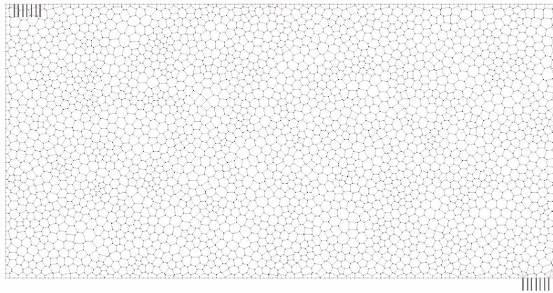
This example shows [Schw04] a net where water is filled in steadily from the entrance in the upper left corner and moves into the lower right corner. Obviously, this net does not consist of triangles or quadrangles, but it is a decomposition of any convex polytope cells. The net was generated by a voronoi decomposition and voronoi cells are used as the basis for the FEM.
