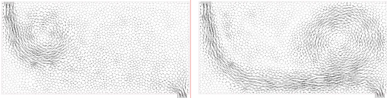
These pictures show the results of the FEM simulation, which was done with n-dimensional convex polytope cells. The computation of the linear system was done with the sparse matrix package of Heimsund. After 8 minutes a whirl appeared, which moved to the right side (150 minutes) to build a quasi stationary whirl. The perspective is from above. This is part the current research at the Institute of Computer Science in Civil Engineering in Hannover, Germany.
