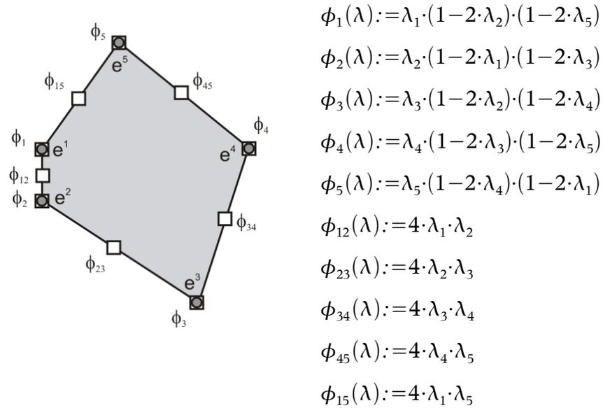
Figure 9: Lagrangian interpolation functions - edge-square
