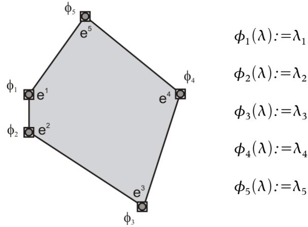
Figure 8: Lagrangian interpolation functions - edge-linear
