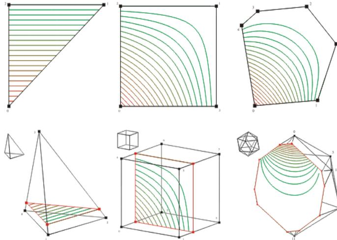
Figure 6: Characteristic of the natural element coordinates in 2- and 3-dimensional convex polyhedrons
