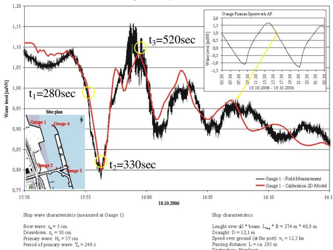
Fig. 1: Ship-Induced Wave System in the Port of Stade-Bützfleth
