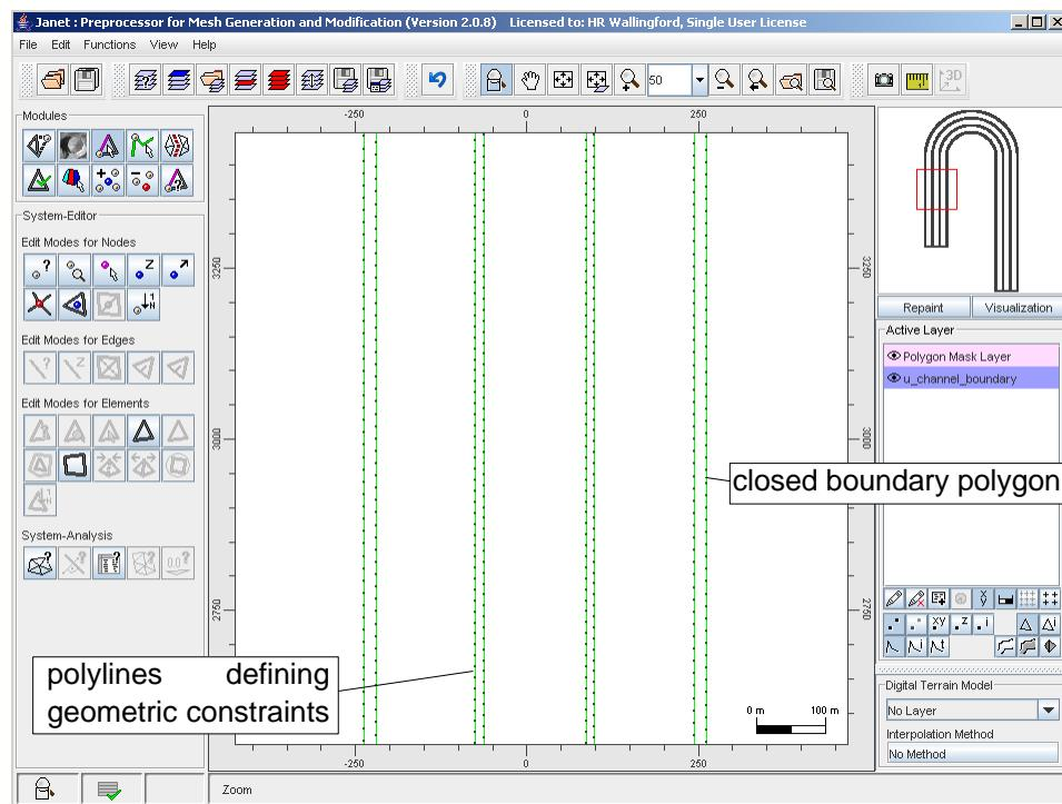
**Figure 2-1.** Boundary polygon and additional polylines
