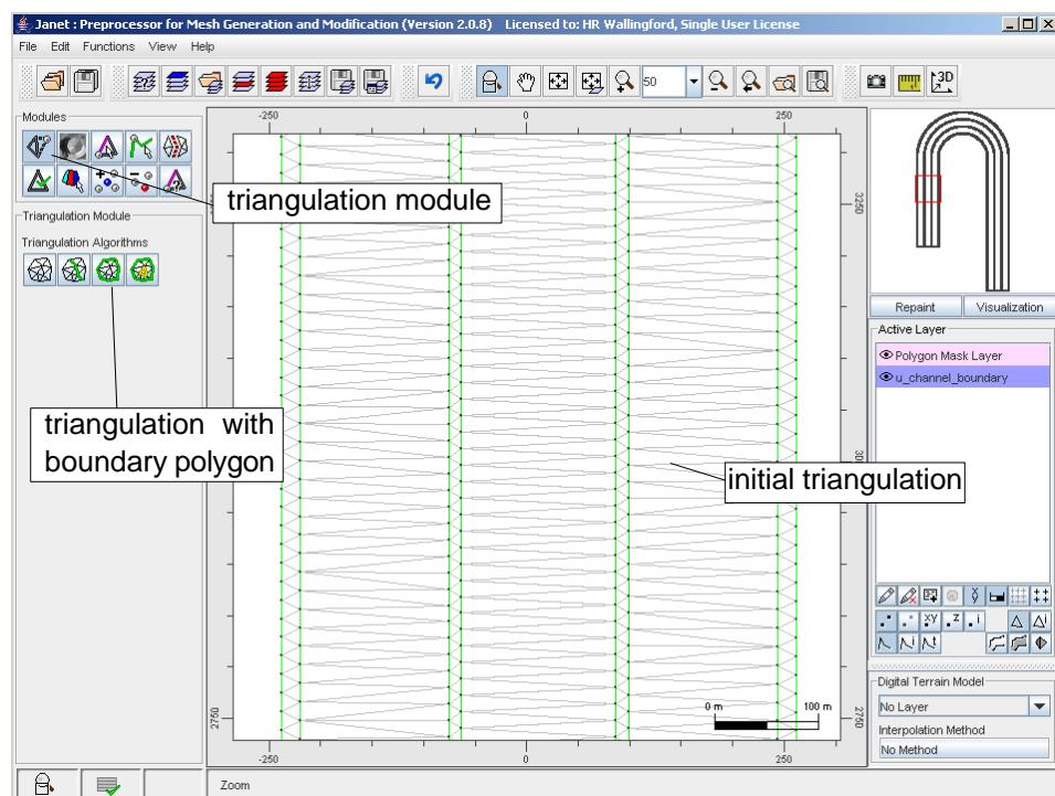
**Figure 2-2.** Boundary polygon and additional polylines
