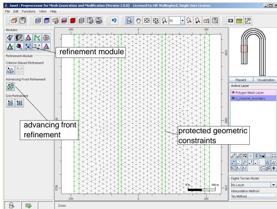
**Figure 2-3.** Boundary polygon and additional polylines
