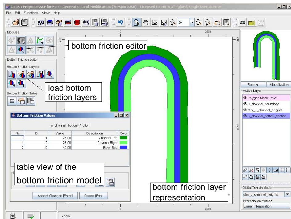
Figure 2-9. Imported bottom friction model
