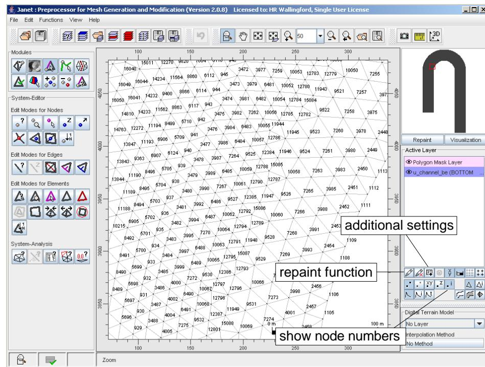
Figure 1-8. Modify visualization settings with quick edit buttons
