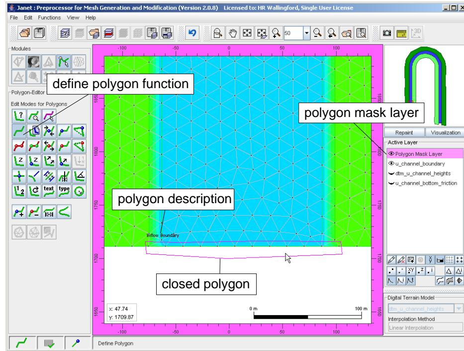
Figure 2-10. Definition of a polygon mask
