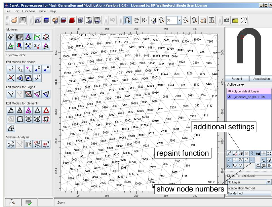
Figure 1-8. Modify visualization settings with quick edit buttons
