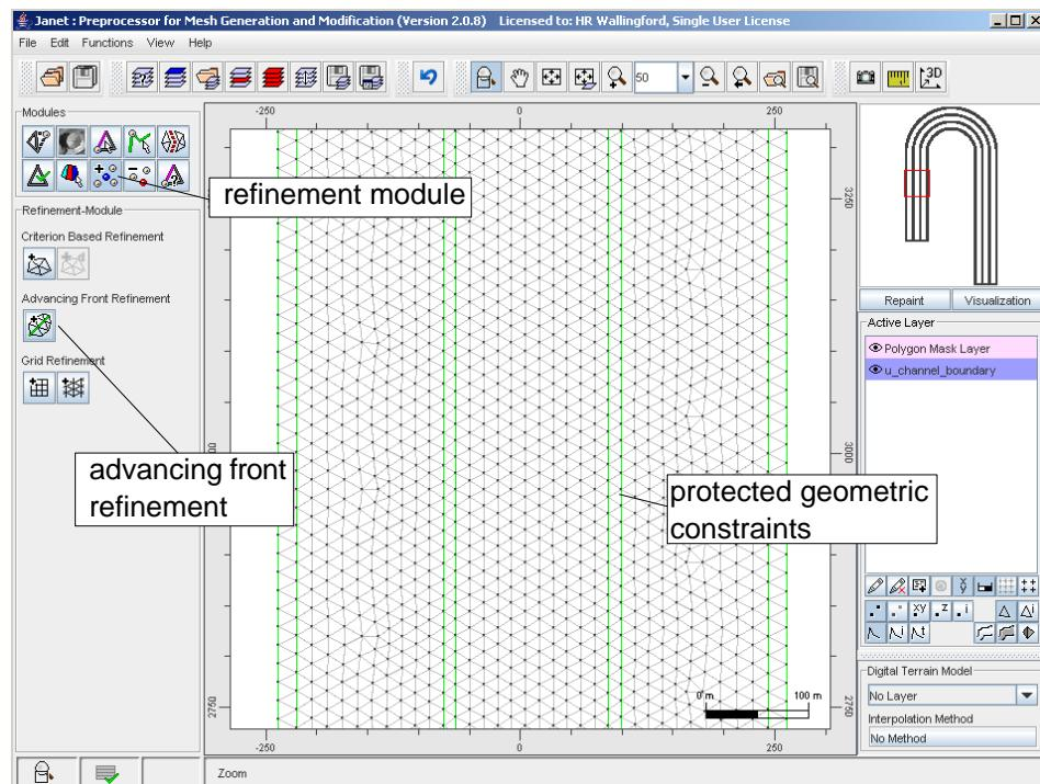
**Figure 2-3.** Boundary polygon and additional polylines
