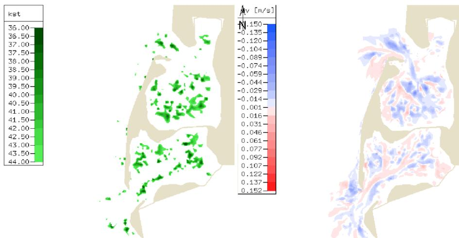
Figure 10. Equivalent friction coefficients for flexible vegetation (left) and velocity differences (right) due to the existence and consideration of seaweeds.
