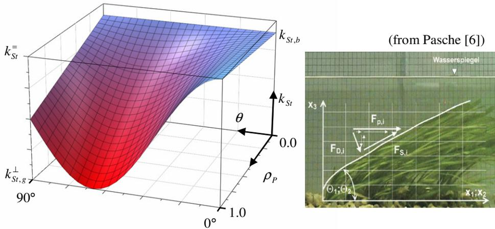
Figure 7. Dynamic equivalent roughness parameters  $k_{St}$  reproduce the flexible behaviour of seagrass plants as additional resistance in hydrodynamic-numerical models.
