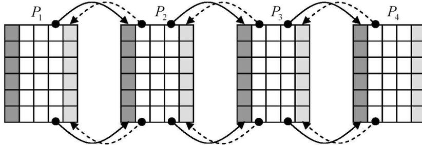
Figure 10: Data decomposition and implementation of the ghost-cell technique
