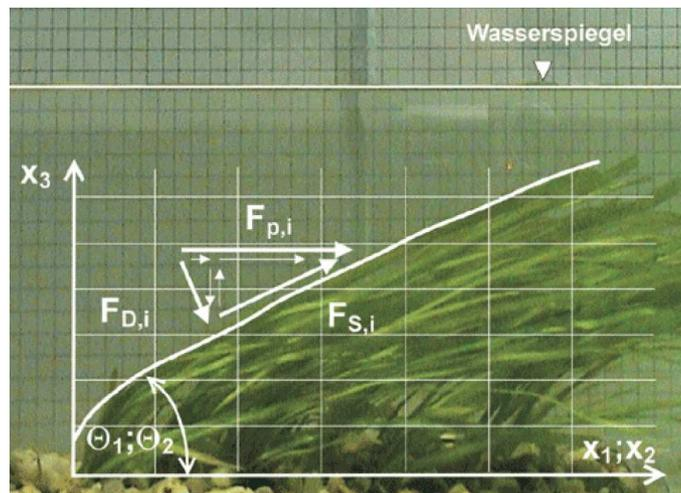
Figure 6: Resistance forces caused by the leaves of seaweeds (see [6])
