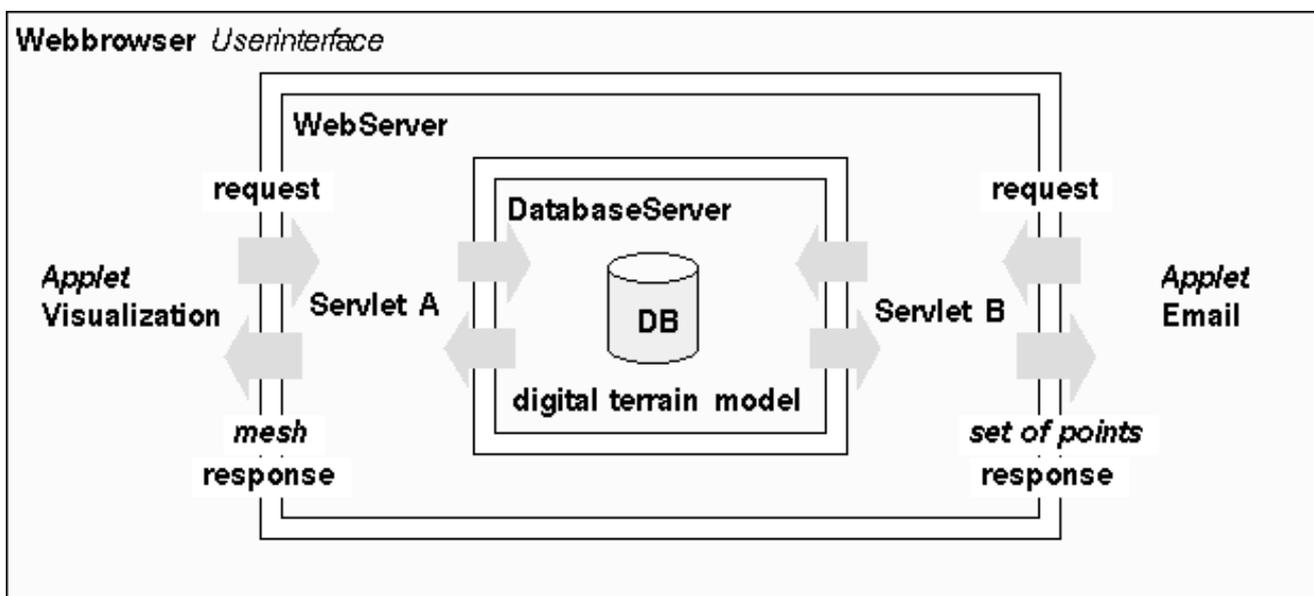
Figure 5: Application of Java applet-servlet technology for distributed grid generation.
