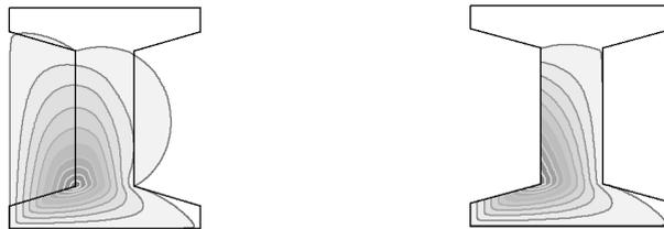
Figure 4: Contour lines of the natural element coordinates
