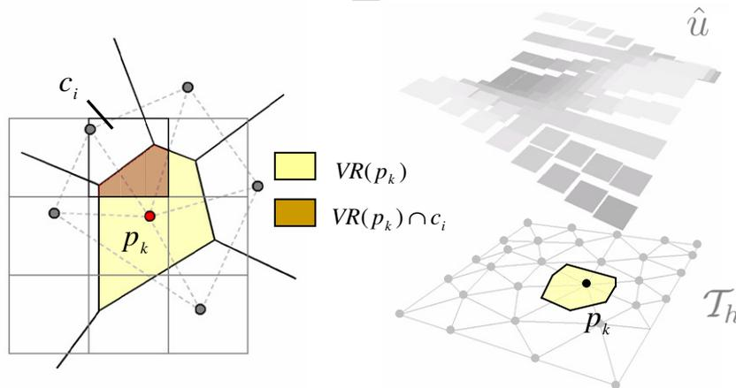
Figure 5. Consideration of all cells  $c_i$  in the voronoi-region  $VR(p_k)$  for FE-Cell coupling.
